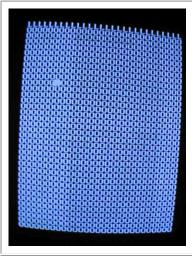
Board will not boot. Screen covered with zeros. Top row changes to different letters and a single object changes in the center as the board tries to boot.
