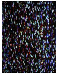
Fast moving short vertical lines covering screen. High pitch squeal from monitor. Caused by shorting 6 MHz clock signal to other chip pins.
