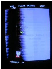
Blue tornado moving quickly from right to left. Can also be a solid blue block with the score and credit ok.
